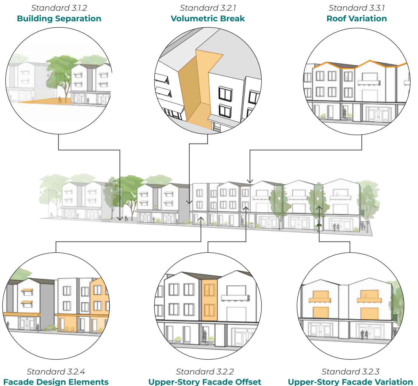
Figure 3-1. Overview of Building Design Standards
